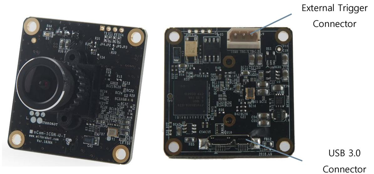
Figure 2. oCam-1CGN-U-T board
