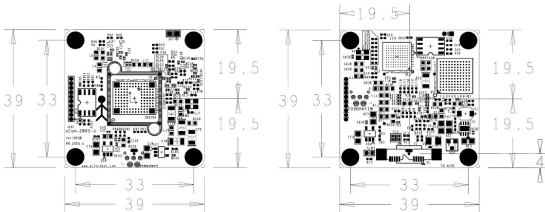
Figure 4. Board size (Unit: mm)
