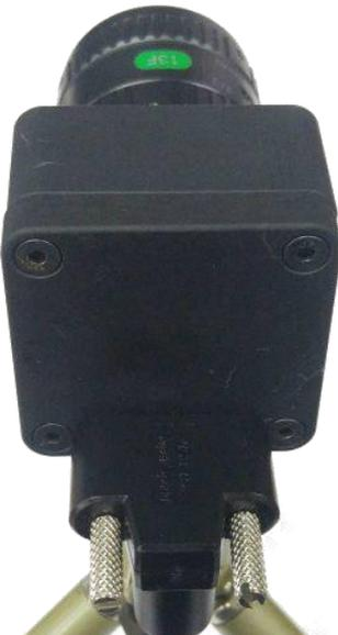
Figure 10. USB 3.0 Connector with Locking Pins
