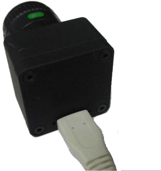
Figure 9. Normal Type USB 3.0 Connector
