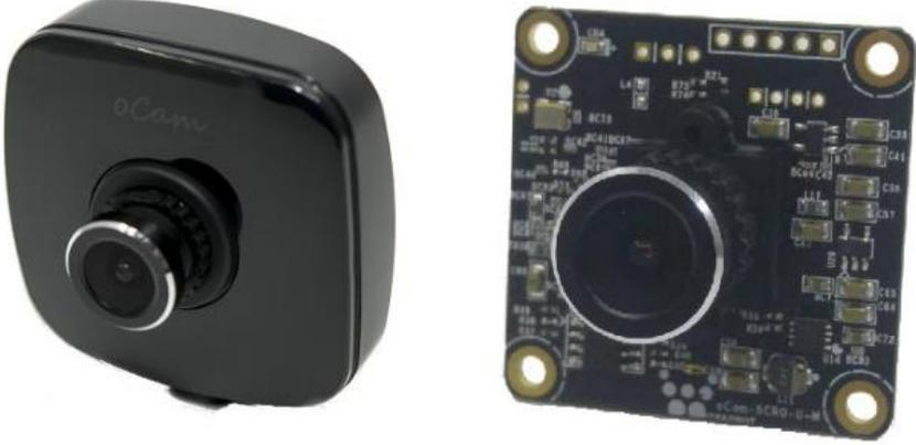
The oCam supports plug-and-play by UVC compliant adapting the standard M12 lens with focal length of 3.6mm. Direct memory access via USB 3.0 allows data to be written to main memory without going through the CPU. It reduces the CPU work load significantly.
