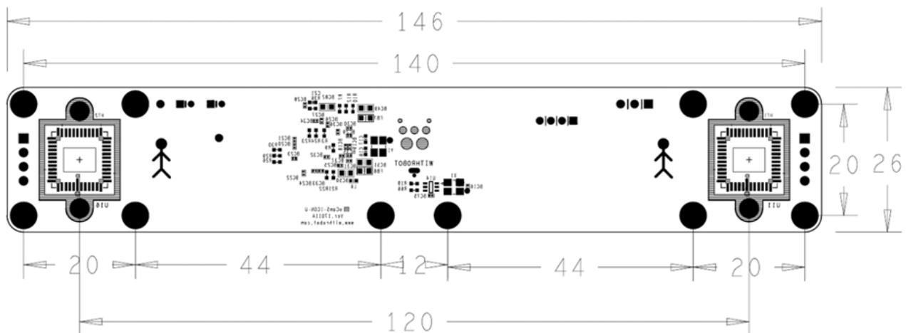
Picture 7. PCB Dimension (unit: mm)
