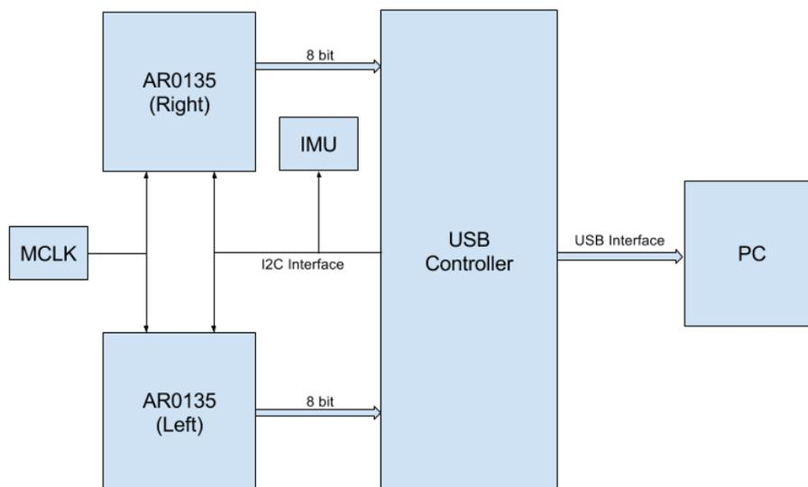
Picture 5. Functional Block Diagram
