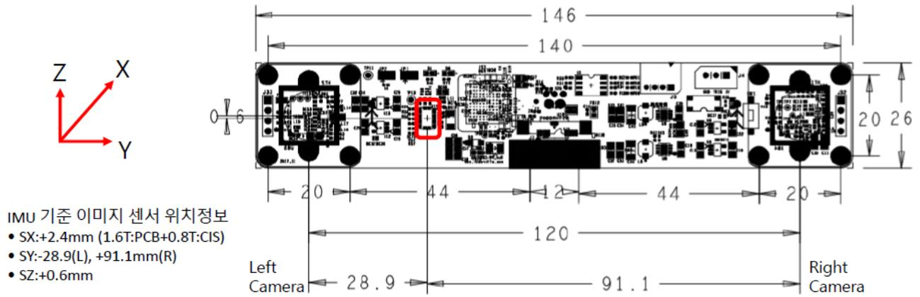
Picture 17. Image Sensor Position with respect to the IMU Sensor
